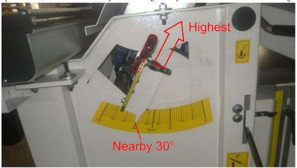
2- Put a wood stick(longer than 1200mm) into the machine, across the belt press on the saw motor pulley.
