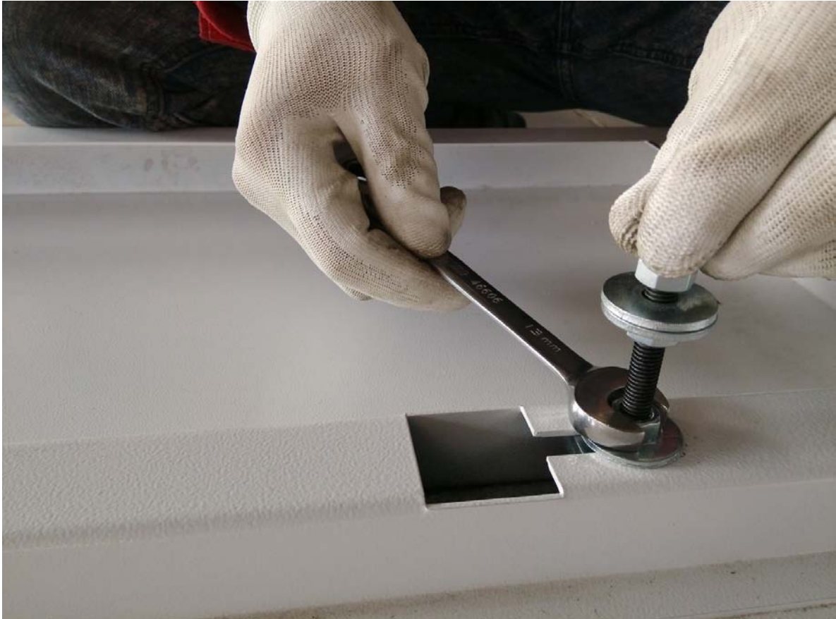
4- Assemble extension working table ,adjust 40*40 Aluminum square rail.
