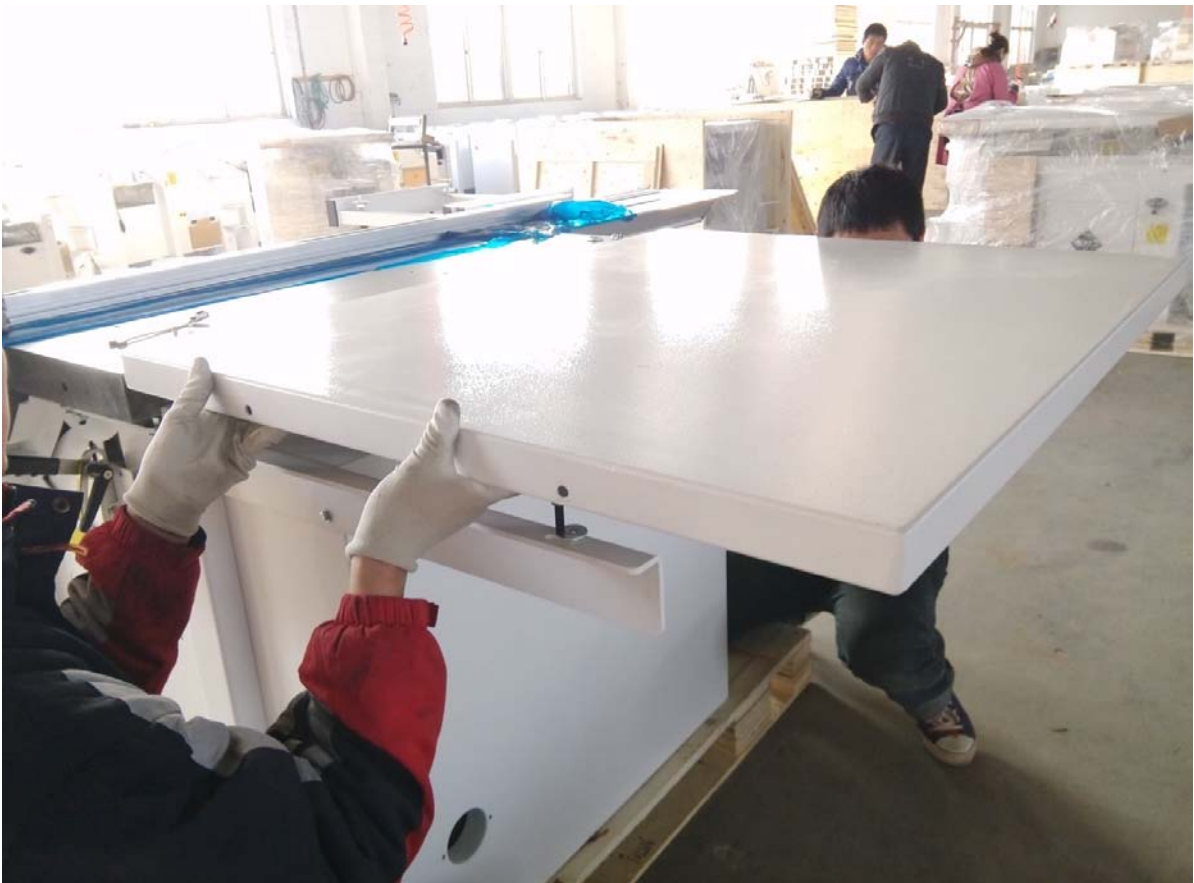
4- Assemble extension working table ,adjust 40*40 Aluminum square rail.
