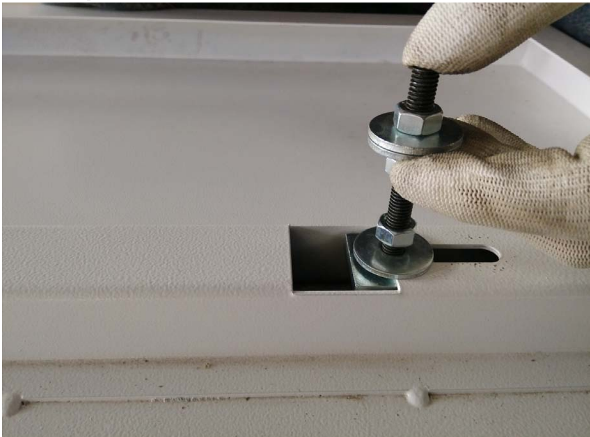
3- Assemble the square screw
